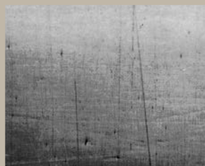
下みがき不十分による研磨キズ Seam and pinhole texture at crossing by less foregoing polish
