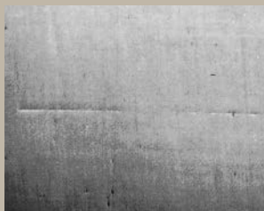
研磨圧力高すぎによる研磨キズ残存 Scratch remains due to overload.
