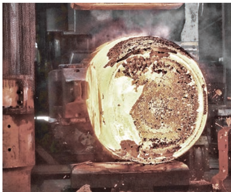
Forging of ESR blocks on the 30MN press ▲
