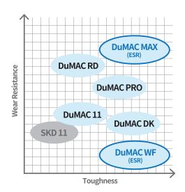
DuMAC series has improved mechanical properties suitable for various and severe usage environments. It provides various options to customers ranging from ESR grades for cutting AHSS to Matrix HSS for punch dies.
